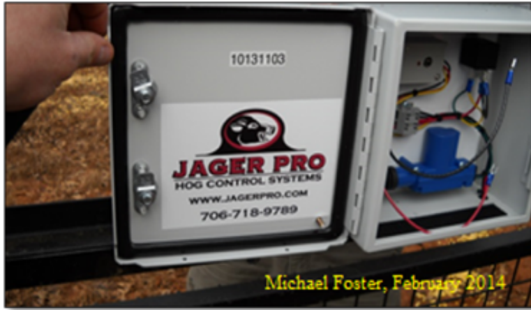
Figure 2.22. Commercial trap door trigger control box. Example from Jager Pro for illustration only. Use does not imply endorsement.
