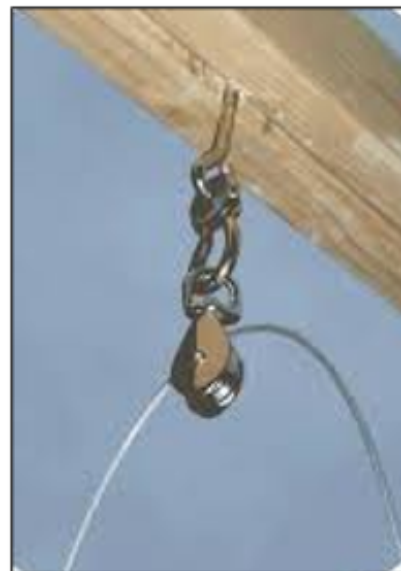
Figure 2.19. A pulley and S hook used for guillotine gates.
